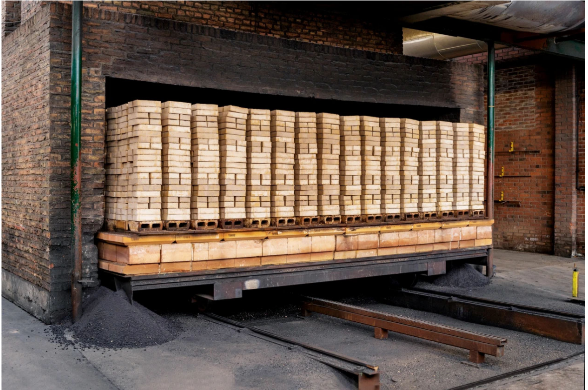
The bricks are taken out of the kiln © Jan Sondergaard
